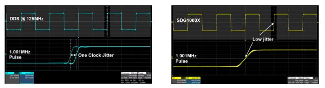
When a Pulse waveform is generated by a common DDS generator, there will be a one-clock-jitter if the sampling rate is not an integer-related multiple of the output frequency. SDG1000X EasyPulse technology successfully overcomes this weakness in DDS designs and helps to produce low jitter Pulse waveforms.
