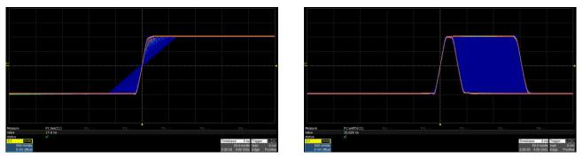
The rise/fall times can be set independently to the minimum of 16.8 ns at any frequency and to the maximum of 22.4 s. The adjustment step is as small as 100 ps. The Pulse width can be fine-tuned to the minimum of 32.6 ns with the adjustment step as small as 100ps.
