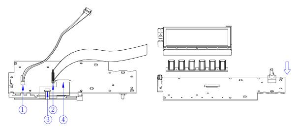
9. Remove all the 9 screws affixed to the power supply board using the T10 Torx screwdriver. Separate the power supply board carefully from the main body of the generator in order to avoid being scratched by the sharp metal edge.
