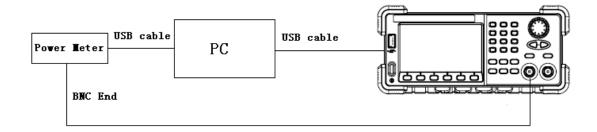
3. Select Sine waveform of the generator and set the amplitude to 0.5 Vpp and frequency to the values listed below in sequence.
