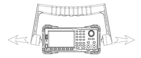
2. After removing 4PCS screws of the pad and 1PCS screw at the bottom of the generator's case, remove the metal shell carefully from the main body to avoid being scratched.
