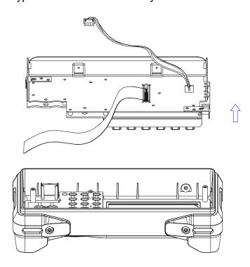
7. Remove the 3PCS screws holding the screen bracket and remove the metal front panel.
