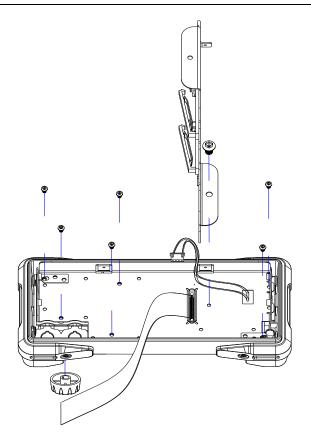
6. Remove the keypad circuit board assembly.
