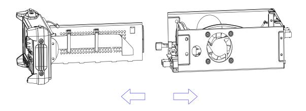
5. Pull out the knob and then remove the screws attaching the hardware partition plate and the front cabinet screws.
