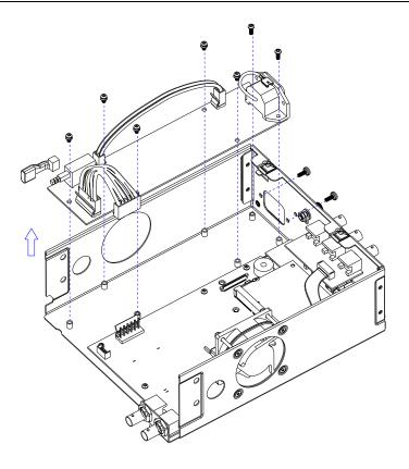
10. Pull out the connecting cable as shown in the following figure and then remove the fan, rear interface board, channel board and main board.
