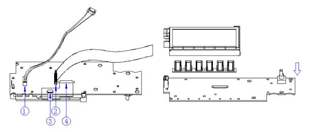
9. Remove all the 9 screws fixed the main board and power supply board using the T10 Torx screwdriver and separate the main board and power supply board carefully from the main body of the generator to avoid being scratched by the sharp metal edge.
