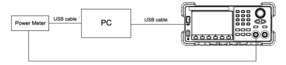
3. Select Sine waveform of the generator and set the amplitude to 1 V and then step through the frequencies listed below in sequence. Then, set the amplitude to 2.5V and repeat the frequency steps.
