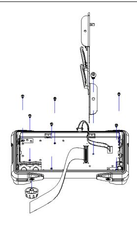
6. Remove the keypad circuit board assembly.
