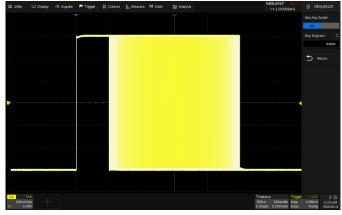
Segmented memory collection will store the waveform into multiple memory segments (up to 80,000) and each segment will store a triggered waveform as well the dead time information. The interval between segments can be as small as  $1.3 \,\mu$ s. All of the segments can be played back using the History function
