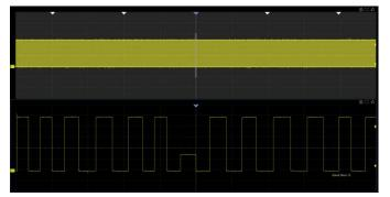
The oscilloscope can search events specified by the user in a frame based on hardware. Events flagged by the Search can be recalled automatically using Navigate. It can also navigate by time (delay position) and history frames
