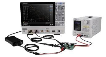
The oscilloscope can control the isolated USB AWG module or a stand-alone SIGLENT SDG generator, to scan the amplitude and phase-frequency response of the DUT, and display the data as a Bode Plot. This makes it possible to replace expensive network analyzers in some applications
