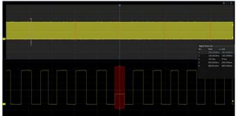
SignalScan automatically searches events by software according to the search conditions set by users, and marks them. Different from hardware search, in SignalScan the supported search conditions are richer, while the scan speed is relatively slower
