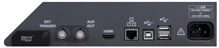
USB Host 3.0 x2, USB Host 2.0 x2, USB Device 2.0 (USBTMC) x1, LAN (VXI-11/Telnet/Socket) x1, micro SD card x1, Auxiliary output (Pass/Fail, Trigger Out) x1 and HDMI x1
