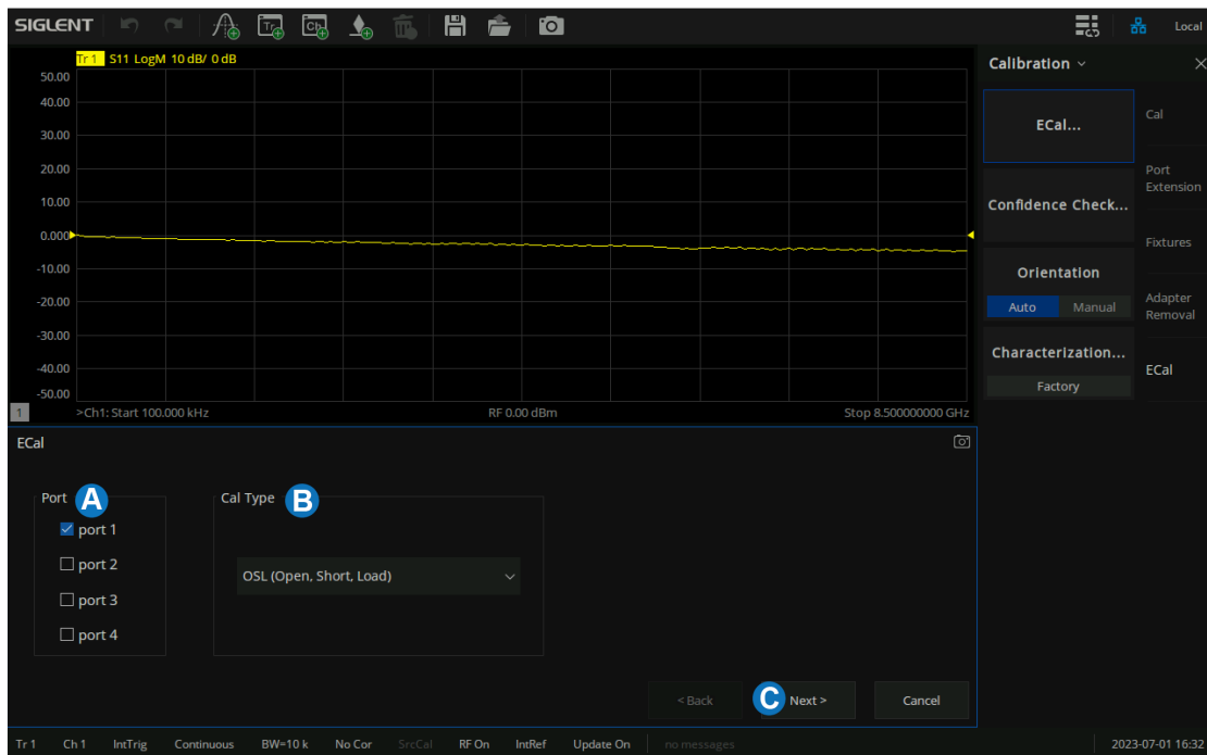
Figure 7-16 ECal config menu
