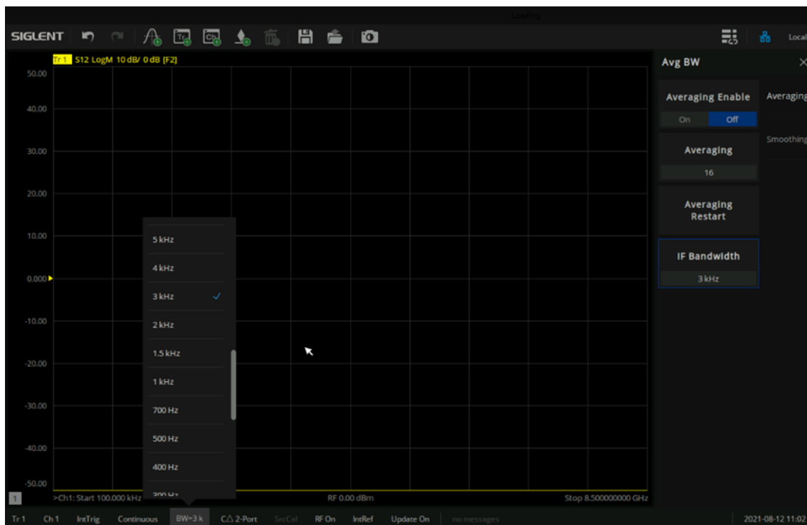
Figure 6-9 Set the IF from the status bar
