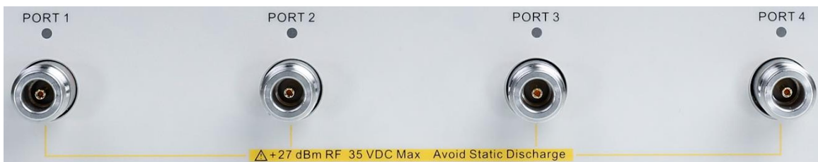
Figure 5-6 Front panel RF connectors (4-port VNA)
