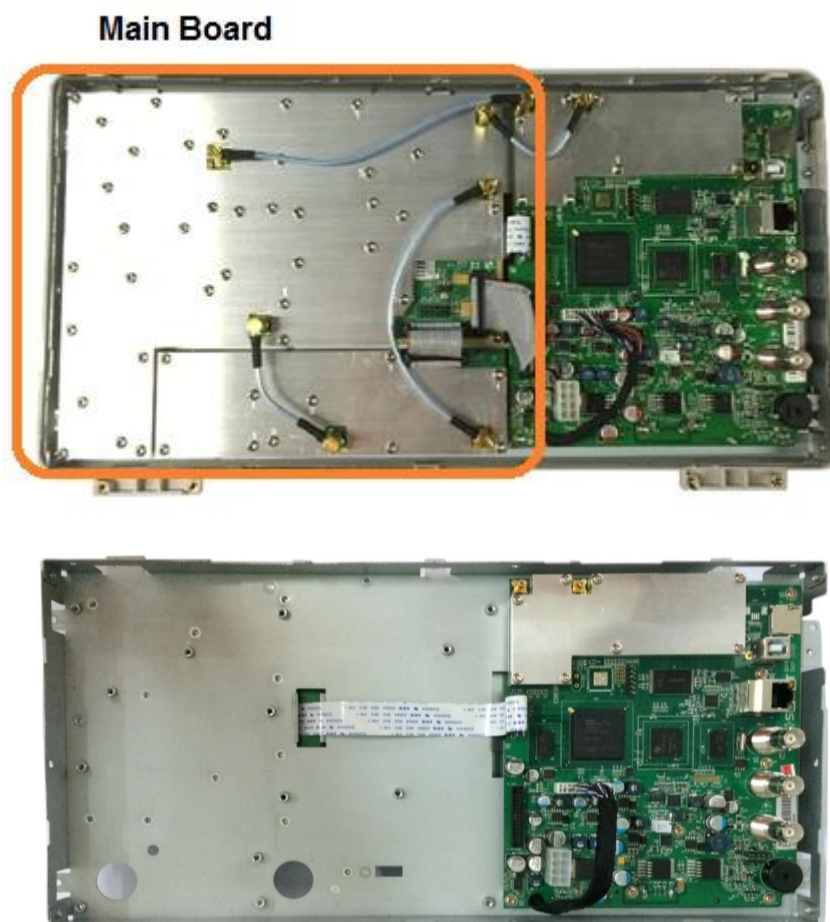
Figure 4-4 View of front panel subassembly with main board (upper) and with main board removed (lower)
