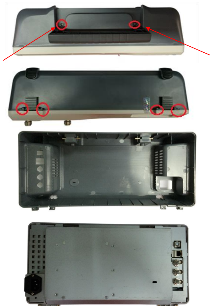
Figure 4-1 Removing the Rear Panel Screws
